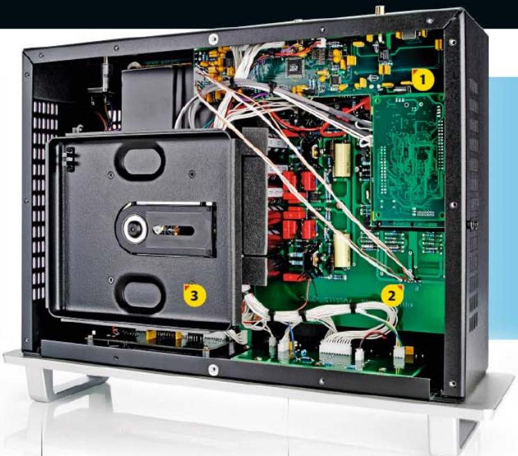
DAC and, just like those, the CD6 uses four 24-bit DACs per channel and dual master oscillators - one to govern 44.1/88.2/176.4kHz sampling rates and the other for 48/96/192kHz. This helps give the most accurate digital timing, leading to better sound quality.
